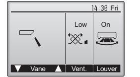
Indoor unit fan may operate even when the ventilation unit is operated individually, depending on the models of the indoor unit and the ventilation unit.
